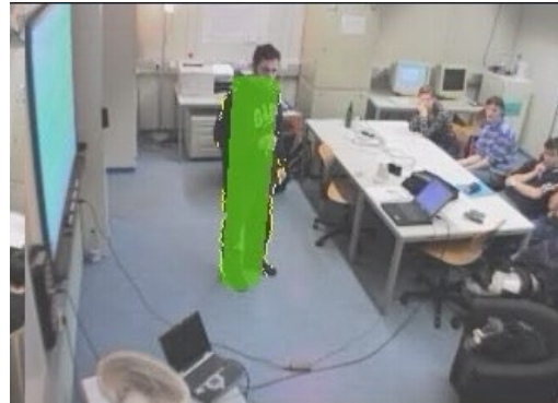
Figure 5: A single camera view showing the projected cylinder model (green) and found edge pixels (white).
