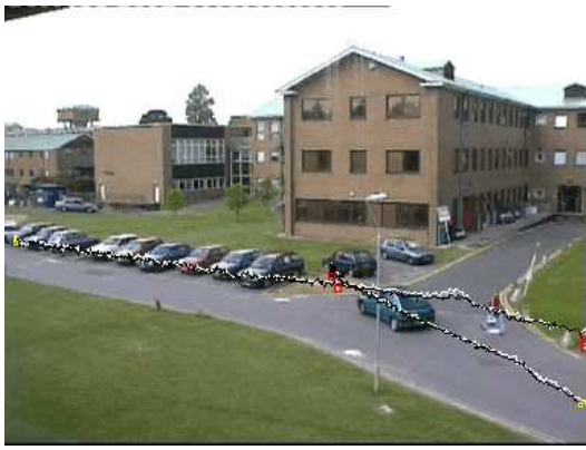
Fig. 8. A comparison of estimated tracks (black) with ground truth positions (white), for two tracks superimposed on a mid-sequence frame showing the two objects.
