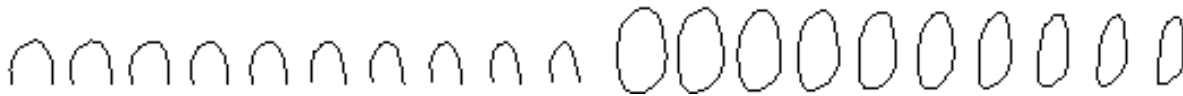
Figure 2: Snake models for u and o features showing the major mode of variation.
