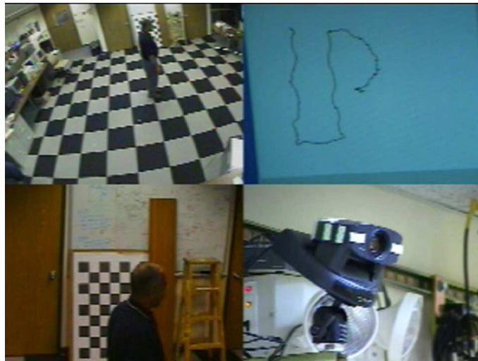
Figure 1.5. The active head tracker. Top left: a person seen by one of the fixed, wide-angle cameras. Bottom left: a close-up view captured by the PTZ camera (seen bottom right). Top right: the track of the person's head projected into the horizontal plane.
