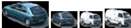
Figure 1.2. Appearance models from a PETS 2001 video sequence, showing the appearance of model pixels, as one model recedes (left) and another approaches (right). Pixels not in the model appear black.
