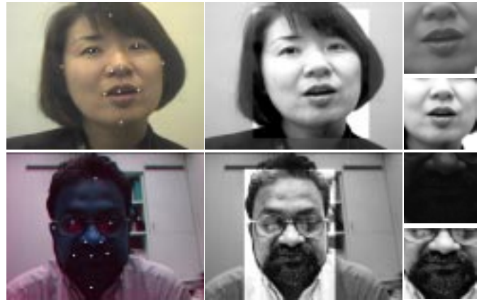
Fig. 2. Face, facial part detection, and ROI extraction for example video frames of two subjects recorded at a controlled studio environment (upper row) and in a typical office (lower row). The following are depicted for each set (left to right): Original frame with eleven detected facial parts super-imposed; face-area enhanced frame; size-normalized mouth-only ROI (upper); and size-, rotation-, and lighting-normalized, enlarged ROI (lower).
