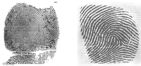
Fig. 1 Rolled inked fingerprint (left), fingerprint acquired with CMOS sensor (right).
